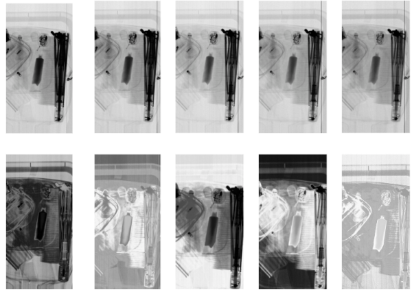
Fig. 3: Comparison between raw spectral bands (top row) and UMAP-projected bands (bottom row).
