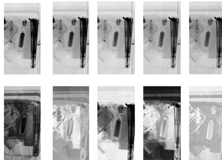
Fig. 3: Comparison between raw spectral bands (top row) and UMAP-projected bands (bottom row).
